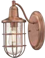
• 65806 Crestview Wall Fixture Washed Copper Finish Clear Seeded Glass Height: 12.25" Width: 5.50" Extends: 9.75" Height from Center of Outlet Box: 6.50" Back Plate: H: 9.06" W: 5.39" Use (1) Medium (E26) Base Lamp, 60W Maximum
