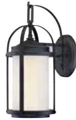
• 65799 Grandview Wall Fixture Matte Black Finish Frosted Glass Height: 17.00" Width: 7.25" Extends: 10.00" Height from Center of Outlet Box: 8.00" Back Plate: D: 6.50" Use (1) Medium (E26) Base Lamp, 60W Maximum
