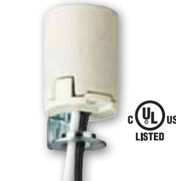
70419 Porcelain Socket Candelabra Base 10" Wire Leads Height - 1 7/8" Diameter - 1" 1/8-IP Hickey 18 Gauge, 105° Leads 75 Watts Max. 125 Volts
