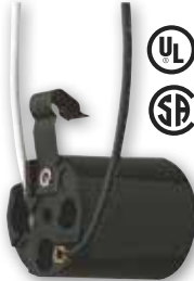
70145 Horizontal Phenolic Snap-In Socket Fits into 7/8" x 1/4" Hole Medium Base 660 Watts Max. 250 Volts
