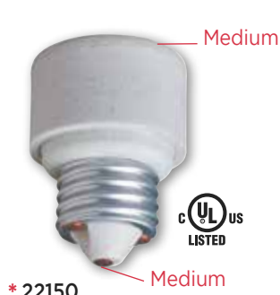
* 22150 70364 Socket Extender Medium Base 660 Watts Max., 250 Volts Extension - 1/4" Overall Length - 2 1/4"
