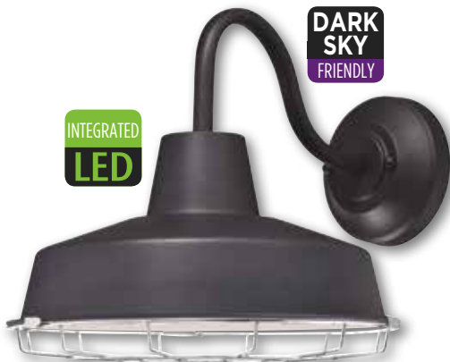
† 62047 Academy 1 Light LED Wall Fixture Textured Black Finish with Chrome Cage Height: 11.00" Width: 12.13" Extends: 15.13" Height from Center of Outlet Box: 4.13" Back Plate: D: 5.00" Includes 13.4 Watt Integrated LED
