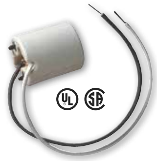
* 22480 High Pressure Sodium Lamp Socket 9" Wire Leads Medium Base SF-2/SEW-2 200° Leads 4 K.V. Pulse Rated 660 Watts Max., 600 Volts 5/32 Screw-Down Height - 1 3/4"
