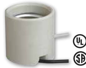
* 22218 Keyless Socket One Screw Surface Mount Medium Base 7" Wire Leads 660 Watts Max., 250 Volts 105° Leads Leads Height - 1 1/8"
