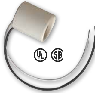
* 22481 High Pressure Sodium Lamp Socket 9" Wire Leads Medium Base SF-2/SEW-2 200° Leads 4 K.V. Pulse Rated 660 Watts Max., 600 Volts 5/32 Bushing Height - 1 3/4"
