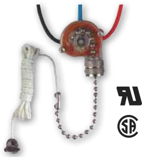
* 22324 - Nickel Finish 3-Way Canopy Switch With 4' White Braided Cord 6" Wire Leads 18 Gauge, 105° Leads Fits 3/8" Hole 1A, 125 VT 3A, 250 VAC 6A, 125 VL 6A, 125 VAC Sequence of Operation: Low / Medium / High / Off Height - 1 3/16" 250V Maximum
