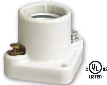
* 22273 One-Piece Receptacle Medium Base 660 Watts Max., 600 Volts Height - 1 1/2" 180° C Maximum Temp.
