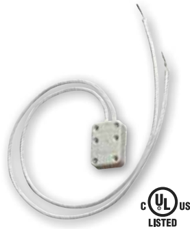
* 22471 Mini BiPin Quartz MR16 Socket GX5.3 Base 12" 18 Gauge Leads SF-1 200° C Leads 100 Watts Max., 250 Volts Height - 1"
