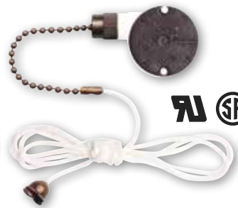
77286 - Single Capacitor, 4-Wire Unit 3-Speed Fan Switch With Antique Brass Pull Chain, 3' Braided Cord 3A, 250 VAC 6A, 125 VAC
