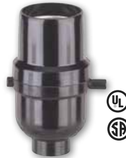
* 22237 Push-Through Phenolic Medium Base 1/8"-IP Cap with Side Screw Aluminum Screw Shell 660 Watts Max. 250 Volts Height - 2 5/8"
