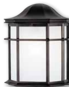
66898 1 Light Wall Fixture Textured Black Finish with White Acrylic Lens Height: 9.88" Width: 7.75" Extends: 4.13" Height from Center of Outlet Box: 4.25" Back Plate: H: 9.38" W: 7.00" Use (1) Medium (E26) Base Lamp, 60 Watt Maximum
