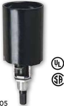
* 22205 1-Piece Phenolic Shell Bottom Turn Knob Socket Medium Base Nipple 1/8"-IP 660 Watts Max. 250 Volts Height - 3 1/4"
