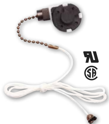
77288 - Dual Capacitor, 4-Wire Unit 3-Speed Fan Switch With Antique Brass Pull Chain, 3' Braided Cord 3A, 250 VAC 6A, 125 VAC
