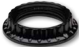
70435 Phenolic Shade Ring For Medium Base Sockets Outside Diameter - 2 3/16" Inside Diameter - 1 5/8" For use with phenolic sockets only.
