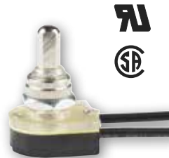
* 22306 Push Canopy Switch 4 3/4" Wire Leads 18 Gauge, 105° Leads Fits 3/8" Hole 3A, 250 VAC 6A, 125 VL 6A, 125 VAC Height - 1 1/4"
