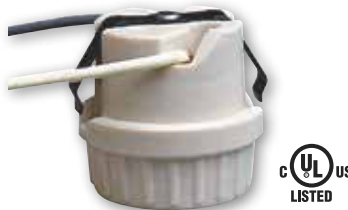
* 22212 70424 Porcelain Snap-In Socket Medium Base Fits 1 1/2" Hole 6" Wire Leads Height - 1 3/4" 18 Gauge, 125° Leads 660 Watts Max. 250 Volts
