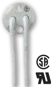
* 11104 Porcelain Halogen Socket 5" Wire Leads SF-1 200° C 300V Leads 100 Watts Max., 250 Volts Fits G4, GX5.3, GV5.3 and G6.35 Lamp Bases Height - 3/8"
