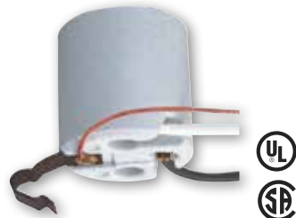
* 22372 Snap-In Porcelain Socket Medium Base 9" Wire Leads Fits 3/8" x 1/4" Hole 18 Gauge, 105° Leads 660 Watts Max., 250 Volts Height - 2"
