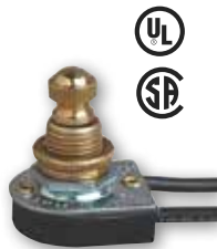
* 22303 - Brass Knob Single Pole Rotary Switch With Removable Knob 6" Wire Leads 18 Gauge, 105° Leads 3/16" Nipple Fits 3/8" Hole 3A, 250 VAC 6A, 125 VL 6A, 125 VAC Height - 1 1/16"
