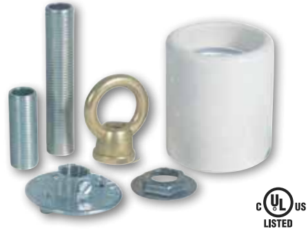
70408 Porcelain Keyless Socket Adapter Kit 1/8-IP Threaded Cap 660 Watts Max. 250 Volts
