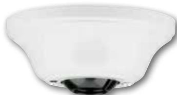
77079 - White Finish Canopy Kit 3 / 4 " I.D. Ball Included Can be mounted onto a cathedral ceiling having up to a 25° angle 100 lb. Load Rating
