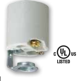
* 22371 70426 Porcelain Fixture Socket Medium Base Height - 2" 1/4-IP Hickey 660 Watts Max. 250 Volts
