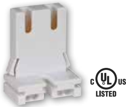
* 22457 Medium BiPin Lamp Holder Floating Action for U-Shape Lamps Low Profile Size 20 Gauge 660 Watts Max., 600 Volts Non Shunted
