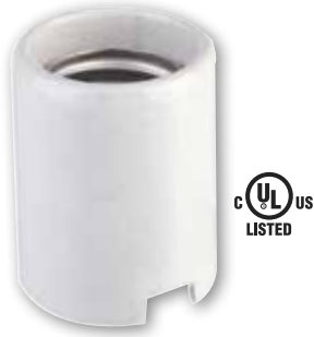
* 22282 Mogul Base Socket 1500 Watts Max., 600 Volts Height - 2 5/8" 4KV Pulse Rating
