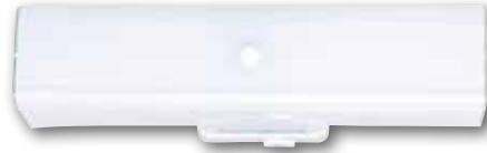
66403 2 Light Wall with Ground Convenience Outlet White Finish Base with White Ceramic Glass Height: 4.50" Width: 14.00" Extends: 5.00" Use (2) Medium (E26) Base Lamps, 75 Watt Maximum
