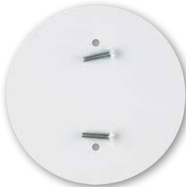
† 29453 - Holes Spaced 2¾" Apart 70064 - Holes Spaced 2¾" Apart Mounts on 3" or 4" Outlet Box † 29452 - Holes Spaced 3½" Apart 70065 - Holes Spaced 3½" Apart Mounts on 4" Outlet Box White Outlet Concealer Diameter - 4¾" Includes: • 2 8-32 x ¾" White Head Screws †Polybagged Bulk Items
