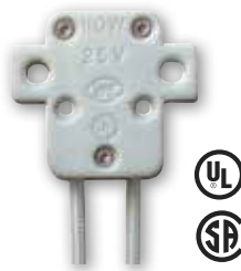
* 11107 MR16 Porcelain Socket 5" Wire Leads SF-1 200° C Leads 75 Watts Max., 125 Volts Fits G5.3, GU5.3 and GX5.3 Lamp Bases
