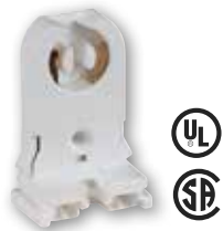
* 22456 Medium BiPin Turn Type Lamp Holder Standard Size No. 18/20 Gauge Panel Mount 660 Watts Max., 600 Volts Non Shunted
