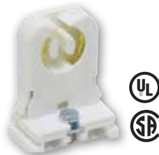
* 22454 Medium BiPin Turn Type Lamp Holder Low Profile Size No. 18/20 Gauge Panel Mount, Captive Mount and Screw 660 Watts Max., 600 Volts Non Shunted
