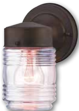
66882 1 Light Wall Fixture Oil Rubbed Bronze Finish with Clear Ribbed Glass Height: 7.50" Diameter: 4.50" Extends: 5.75" Height from Center of Outlet Box: 2.00" Back Plate: D: 4.50" Use (1) Medium (E26) Base Lamp, 100 Watt Maximum
