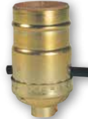
70410 - Brass Finish *22011 - Polished Brass Push-Through Socket with Set Screw On/Off Brass Finish Medium Base Tapped 1/8-IP 660 Watts Max., 250 Volts
