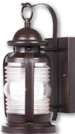
62301 Weatherby 1 Light Wall Fixture Weathered Bronze Finish with Clear Glass Height: 12.75" Width: 6.00" Extends: 7.50" Height from Center of Outlet Box: 7.25" Back Plate: H: 7.88" W: 4.38" Use (1) Medium (E26) Base Lamp, 60 Watt Maximum
