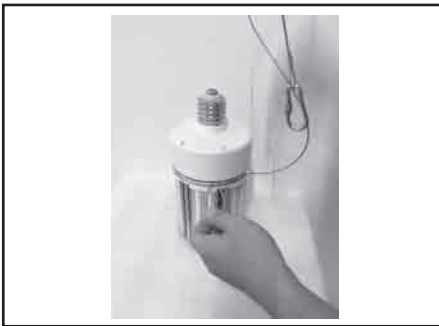
Step 4: Push the safety cable's loop completely through safety cable slot and insert hook end of cable through the loop.
