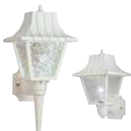
Polycarbonate Wall Fixture with Removable Tail Height with Tail: 17" Height without Tail: 13" Square: 8" Extends: 8.5" Use (1) Medium (E26) Base Lamp, 60 Watt Maximum
