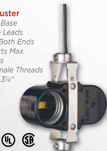
* 22259 Twin Cluster Socket with Male Threads on Each End 6" Wire Leads 18 Gauge, 105° Leads 660 Watts Max. 250 Volts ⅝-IP Nipple Height - 4½"
