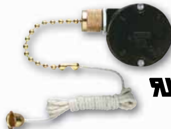
77075 - Triple Capacitor, 8-Wire Unit 3-Speed Fan Switch With Polished Brass Pull Chain, 2' Braided Cord 3A, 250 VAC 6A, 125 VAC
