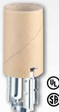
* 22136 3" Keyless Socket Medium Base 1/8-IP Hickey 660 Watts Max., 250 Volts Height - 3"
