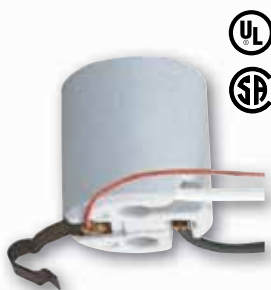
* 22372 Socket Medium Base 9" Wire Leads Fits \frac{3}{8} " x \frac{1}{4} " Hole 18 Gauge, 105° Leads 660 Watts Max., 250 Volts Height - 2"
