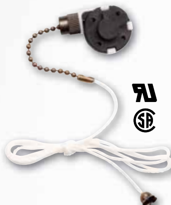
77288 - Dual Capacitor, 3-Wire Unit 3-Speed Fan Switch With Antique Brass Pull Chain, 2' Braided Cord 3A, 250 VAC 6A, 125 VAC
