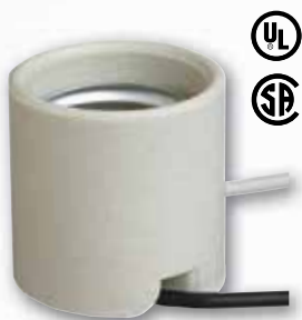
* 22218 Keyless Socket 1 Screw Surface Mount Medium Base 7" Wire Leads 660 Watts Max., 250 Volts 105° Leads Leads Height - 1\frac{5}{8} "
