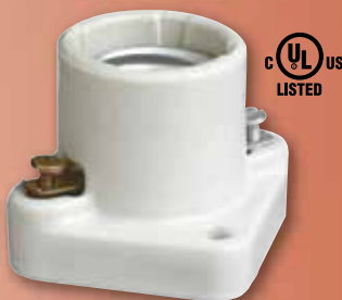
* 22273 One-Piece Receptacle Medium Base 600 Watts Max., 250 Volts Height - 1\frac{1}{2} " 180° C Maximum Temp.
