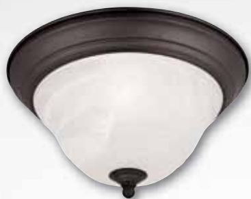
62203 Wensley 1 Light Flush Oil Rubbed Bronze Finish with White Alabaster Glass Height: 6" Diameter: 11.25" Use (1) Medium (E26) Base Lamp, 60 Watt Maximum
