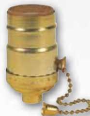
70411 - On/Off 250 Watts Max., 250 Volts 70431 - 3-Way 250 Watts Max., 250 Volts Pull Chain Socket Brass Finish Medium Base Tapped 1/8-IP
