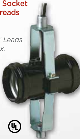
* 22256 3 Light Cluster with Male Threads on Each End 6" Wire Leads 18 Gauge 105° Leads 660 Watts Max. 250 Volts ⅝-IP Nipple Height - 4¾"
