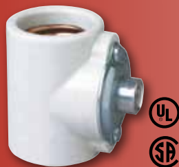
* 22274 Keyless Twin Socket Medium Base Bushing \frac{1}{8} -IP With Set Screw 660 Watts Max. 250 Volts Height - 2\frac{1}{8} "
