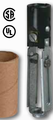
* 22127 70402 (Carded 2-Pack) Adjustable Keyless Socket Candelabra Base 1/8-IP Threaded Hickey 75 Watts Max., 125 Volts Height Adjustable from 3 1/4" - 4 3/4"
