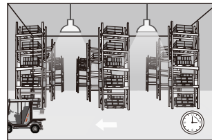
After hold time, the sensor dims the lamp to a low light level if no new motion is detected in its detection zone.
